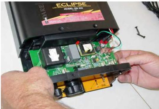
5. Slide inner guts back into place. Replace both screws. Do not over tighten. Turn on energizer, test with a volt meter, you should get a reading above 5,000 volts.
