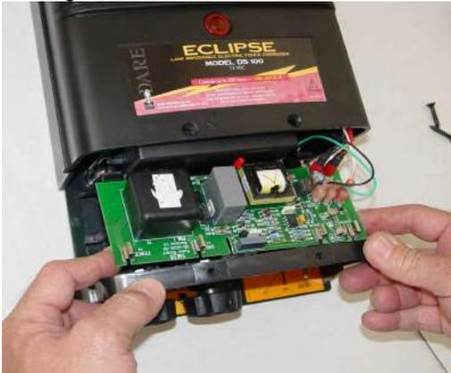
3. Most repairs need to be made by replacing the circuit board. Firmly lift the front of the circuit board up and away from the tabs holding it in.
