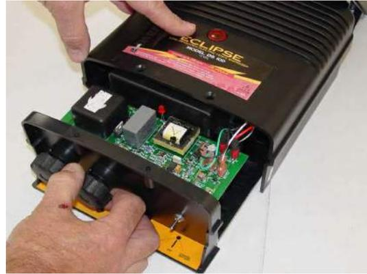
2. Hold down energizer with one hand then slide out inner module by pulling on knob near center.
