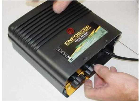
2. Hold down energizer with one hand then slide out inner module by pulling on knob near center (do not pull on power cord).
