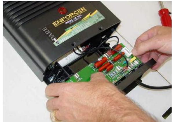
4. Most repairs need to be made by replacing the circuit board. Firmly lift the front of the circuit board up and away from the tabs holding it in.
