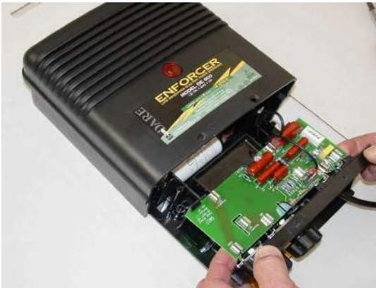
3. Inspect all the components looking for visual damage such as burned areas or cracker parts due to lightning.
