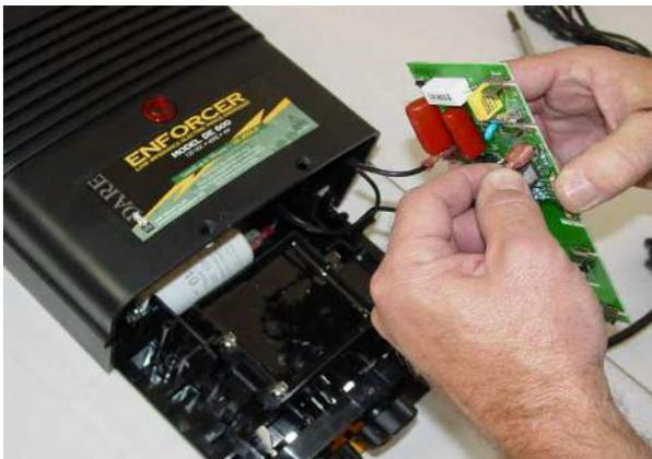
5. Remove the wires from the board one at a time Attaching each to the new board in the same location as you proceed. Continue with all wires. Snap the new board back into place, making sure the light bulb will be seen through the red lens. Plug in the unit and test with a volt meter. You should get a reading above 5,000 volts.
